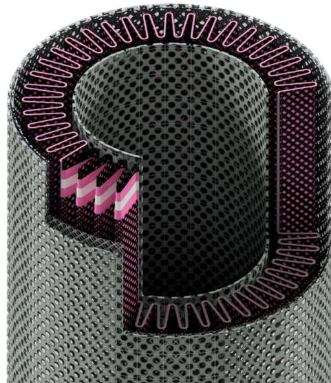
Ultrafine fiber medias were evaluated in conjunction with support materials. By combining ultrafine, moderate, and course fiber layers, overall media integrity was increased, media void volume was enhanced, and pore structure was maintained. When pleated in cartridge form, the element displayed enhanced filtration qualities in high viscosity oils.
