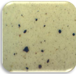
Patch Test Results Brand New Oil In Tote (Before Filtration) ISO 21/19/17
