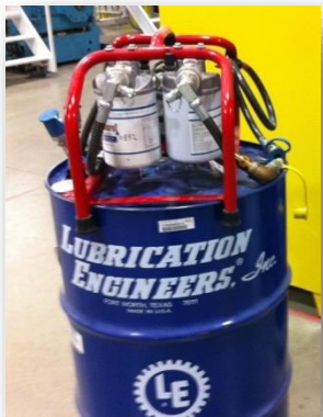
Drum Topper Used To Filter and Dispense New Oil From 55 Gallon Drums Courtesy of Lubrication Engineers®
